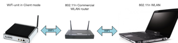
Figure 2.2 – Connection to PC by access point (router)
