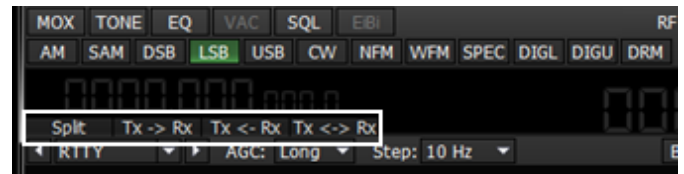
Figure 8.4 – Places on the panel, responsible for frequency exchange between VFO-A and VFO-B
